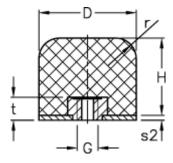
D = 80 t = 12d2 = 3 G = M12 H = 63 Load capacity F (kN) = 60.0 Load capacity f (mm) = 35 Load capacity W (J) = 560 r = 18.0
